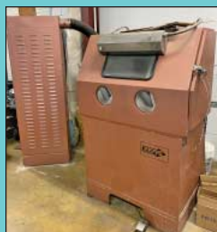
42" Zero Peen Model 55-6-300-R-DF Blast Cabinet w/ Dust Collectors
