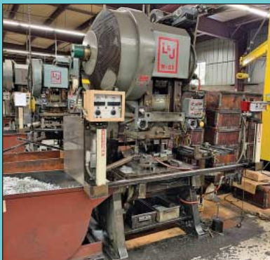
60 Ton L&J Model W-60 Flywheel Type OBI Press
