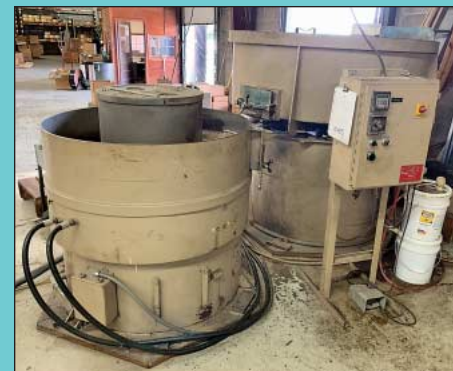
64" Dia. Rosemont Vibratory Bowl Finisher
