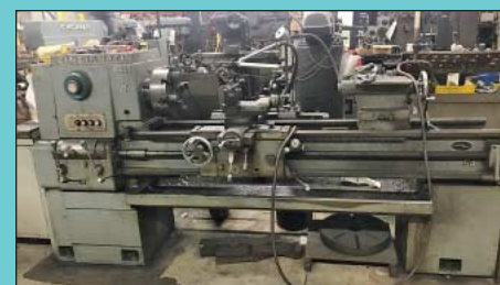
18" x 54" Cincinnati Tray Top Toolroom Lathe w/ Taper Attachment & 12" Chuck
