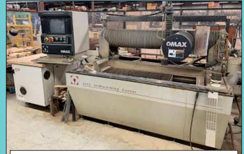
26" x 52" Omax Model 2652 Waterjet Cutting Machine
