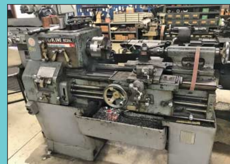
15" x 30" Leblond Regal Toolroom Engine Lathe w/ DRO
